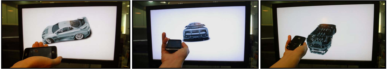
Fig. 1. Mobiature working prototype. A 3D model on a large display is aligned dynamically with respect to the orientation of a mobile device.
